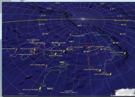
Figure 2. Drifts of the two AITP clusters deployed in April 2008 and August 2008 respectively until October 27, 2008. Red pins represent starting points and yellow pins ending points of the drifts.
