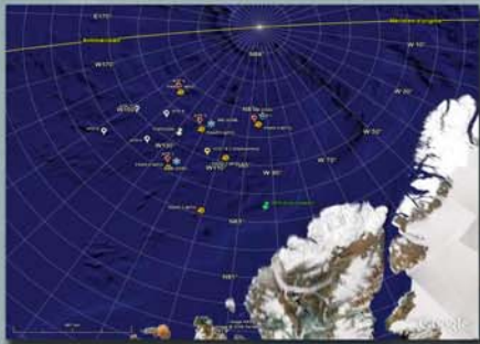
Figure 1. Deployment of the first cluster of 4 AITP (red) + 7 Met buoys (orange) + 3 IMBs (blue) + 2 ULS floats (yellow) in April 2008. Deployment of the second cluster of 4 AITP (white) + one POPS and one IMB in August 2008.
