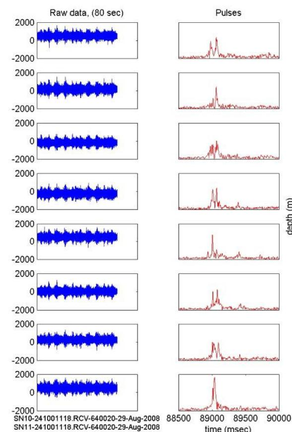
Figure 3 – Acoustical raw data (left) and pulse compression (right) on all 8 channels (from 307 to 979m of depth in 96 m increments).
