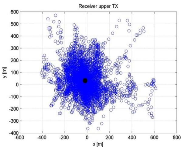
Figure 1 – Scatter of receiver mooring motion at 300m of depth throughout sept 2008- aug 2009.
