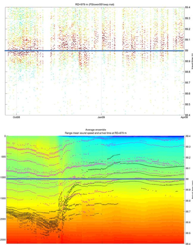
Figure 4 – Measured (upper) and predicted (lower) travel times throughout the experiment. The dots indicate individual arrivals. The color of the dots of measurements indicates the intensity of the arrival. For the predictions black dots represent waterborne arrivals, while pink dots represent bottom interacting arrivals. The colored background of the predictions represent the sound speed field provided by TOPAZ3.
