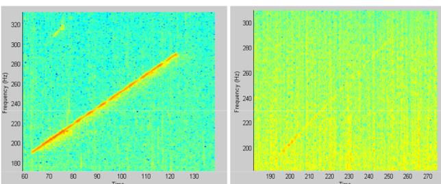
Figure 2 – FM sweep at source (left) and r=60km (right). Duration is 60 seconds and frequencies are from 190 to 290 Hz.
